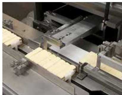
Two phases for portioning and putting into the wrapper infeed chain with lugs
