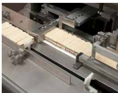
Portioning disk for medium speed applications. Up to 300 cycles/min
