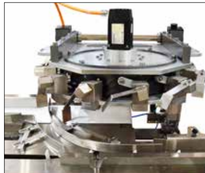
Portioning disk for medium speed applications. Up to 300 cycles/min
